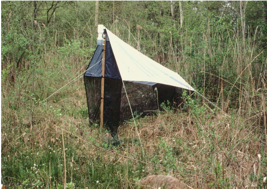
Figure 2. A Malaise trap in use on Frilford Fen
